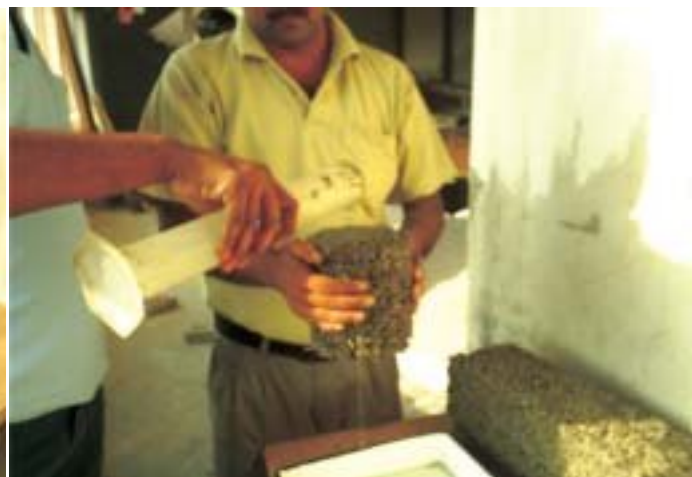
Figure 7: Testing of perviousness of PAVESCAPE Concrete
